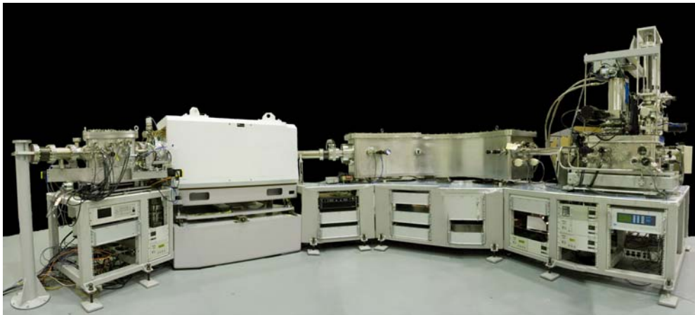
SHRIMP IIe with Multicollector, ready for delivery to Sao Paulo.
